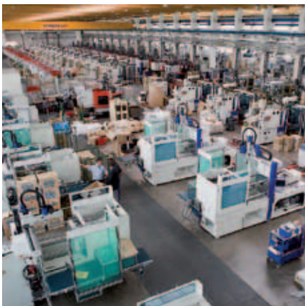
In Dietenhofen, 443 injection moulding machines produce up to 10 million single parts daily.
