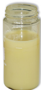
Hydraulic oil with emulsified water
