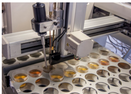
Klotz particle counter with Gilson autosampler CINRG
