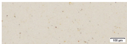
Minimum requirements for new oil according to DIN 51524: Purity class 21/19/16
