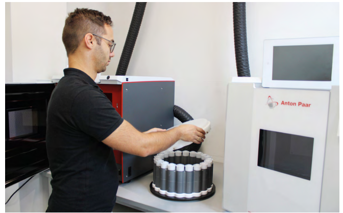
New to the OELCHECK laboratory – two powerful Multiwave 5000 microwave devices from Anton Paar. 20 grease samples are placed on a rotor disc. The microwave devices each require 90 minutes plus 30 minutes cooling time to digest the samples.
